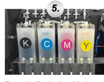
Deeply Optimized Ink Supply System: Smooth Ink Flow, Sufficient Ink Supply, No Printhead Clogging.
